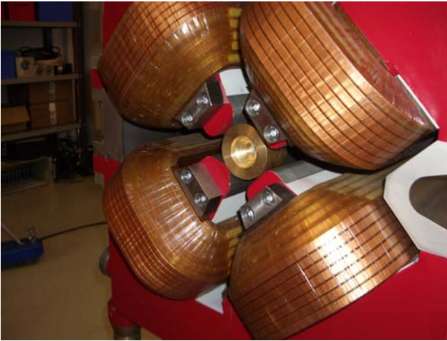
Fig. 4: Inserted mechanical fixture for surveying the geometrical axis of the quadrupole magnet. The fixture is made from brass.
