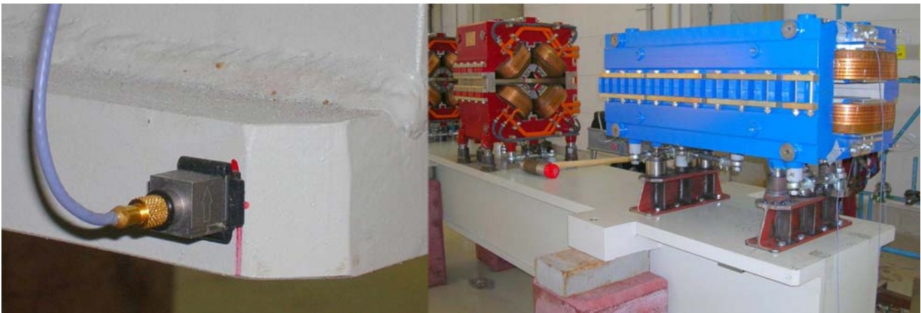
Figure 6: Accelerometer and impact hammer used for modal analysis of girder
