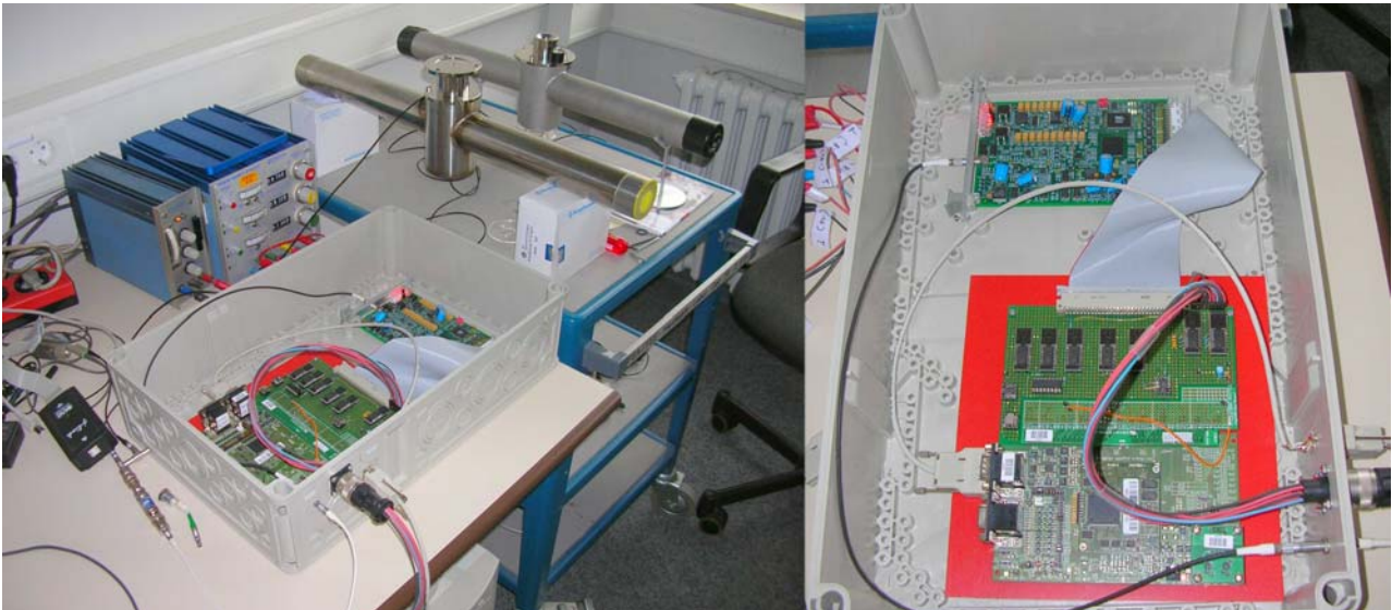
Figure 8: Ultrasonic Hardware for DESY HLS (prototype)
