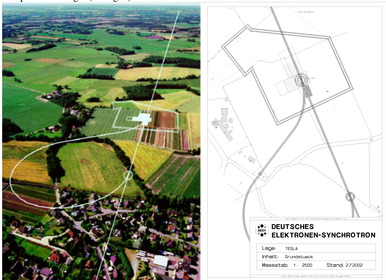
Fig. 2: Visualization and map of main linac and damping ring at a planned construction site
