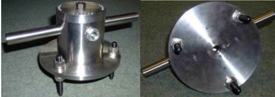
Fig. 7: Photographs of prototypes of new package for ultrasonic sensors
